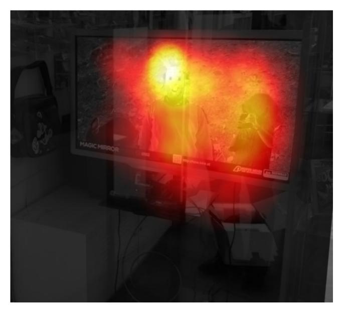
It is possible to utilize the integrated face tracker to output rough estimates for head pose and therefore gaze direction, which can be used to build heatmaps that can - with proper calibration - be overlaid on an image of the actual shopping window. This shows where people generally look at when looking into the shopping window and enhances the shopping window rating with very specific information that is extremely hard to obtain using any other means.
