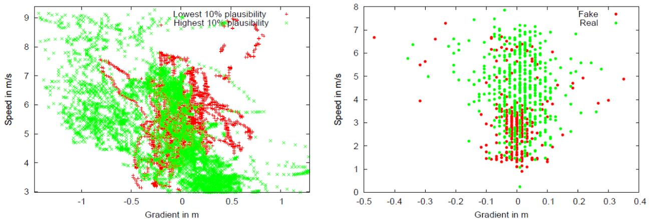
Fig. 4: Left: Scatterplot of gradient vs. speed, coloured by 10% lowest and highest plausibility, on historical data; Right: Same scatterplot on first batch of competition data with by-track user-defined classification Real and Fake.
